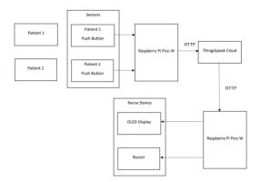
The above block diagram illustrates the emergency alarm system for patients in hospital. The whole system is divided into two parts i.e the device with the push buttons and the device with the nurse. This system uses two Raspberry Pi Pico W's. We have used push buttons for the patients. Whenever they require any kind of emergency
