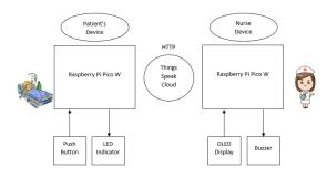
**Raspberry Pi Pico W**: Raspberry Pi Pico W acts as the central processing unit. We have used two Raspberry Pi's i.e one for the Patient and other for the Nurse' device. We have used the Picos with inbuilt WiFi module to connect them on the cloud.
